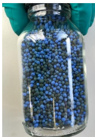
Figure 21 - Formation of two different color spheres after calcination.
